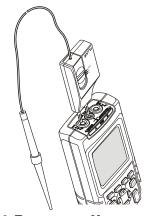
Figure 2-6. Temperature Measurement Setup
