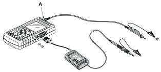
Figure 2-16. Isolated Triggering
